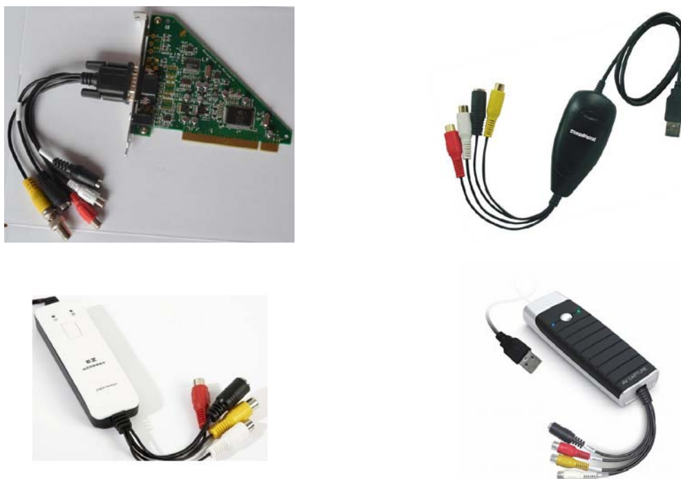
Figure 1: Different types of Video Interface device in common use by members of the NEMETODE team. To the upper left is the Osprey 210 PCI Video Capture Card. Due to its physical size this card requires a full size desktop PC and will not fit in a mid-size or “small form factor” PC chassis. To the upper right is a Climax Digital USB Video Audio Capture Device while the bottom row shows two models of EZ Capture device (discussed in the main text) with Model A on the left and B on the right.
