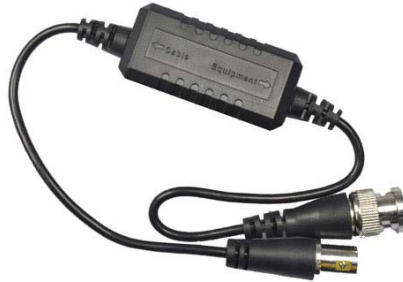
Figure 2: Typical CCTV Ground Loop Isolator. Note the words “Cable” and “Equipment” embossed on the body of the device with “Cable” being the end that leads to the video capture device fitted to the PC and “Equipment” being the end that leads to the camera. Each end has a BNC connector while many cameras, cables and video interface devices have RCA connectors. Search “CCTV BNC RCA adaptor” for converters that allow all items to be connected together.
